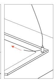
Insert the cables in the holes and then screw the wooden base to the ceiling using a screwdriver (not included). In alternative, use the magnetic fixation. Fine tune the length of the steel cables to level the ViCloud.
